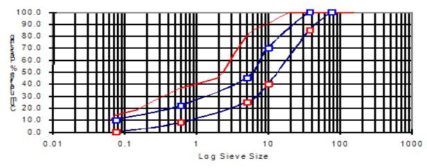
Certified that the Particle Size Distribution was determined in accordance with BS 1377: Part 2: 1990: Method 9.2
